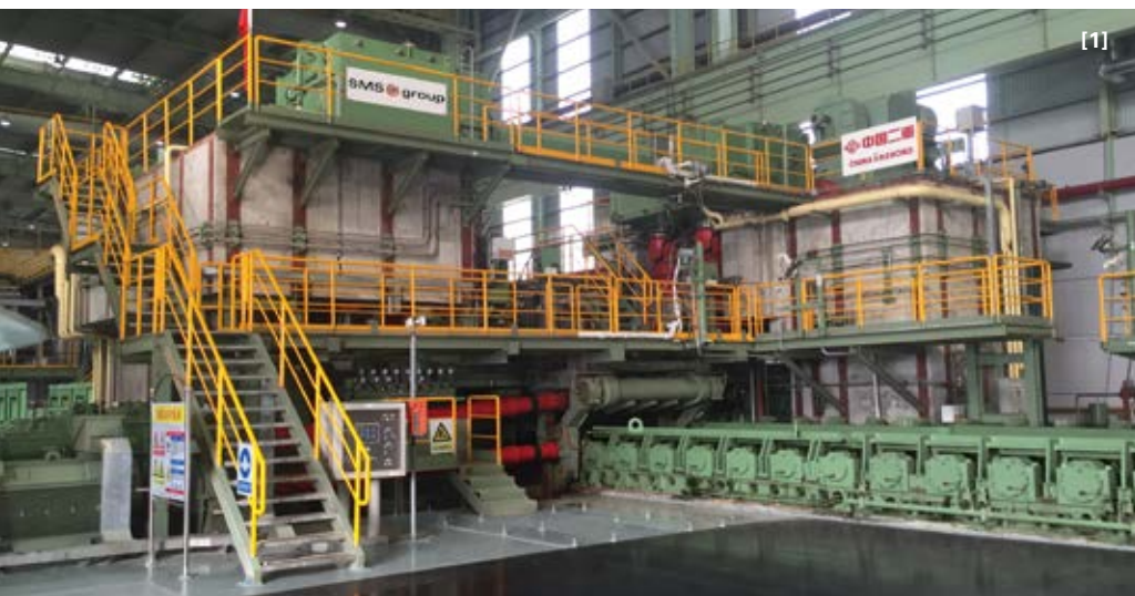
[1] | Slab sizing press. [2] | Coiler. [3] | Four-high reversing stand. [4] | Finishing train.
