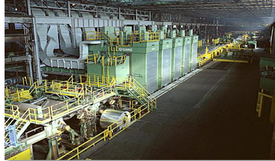
Finishing lines for aluminum hot strip 11 plants since 2000
