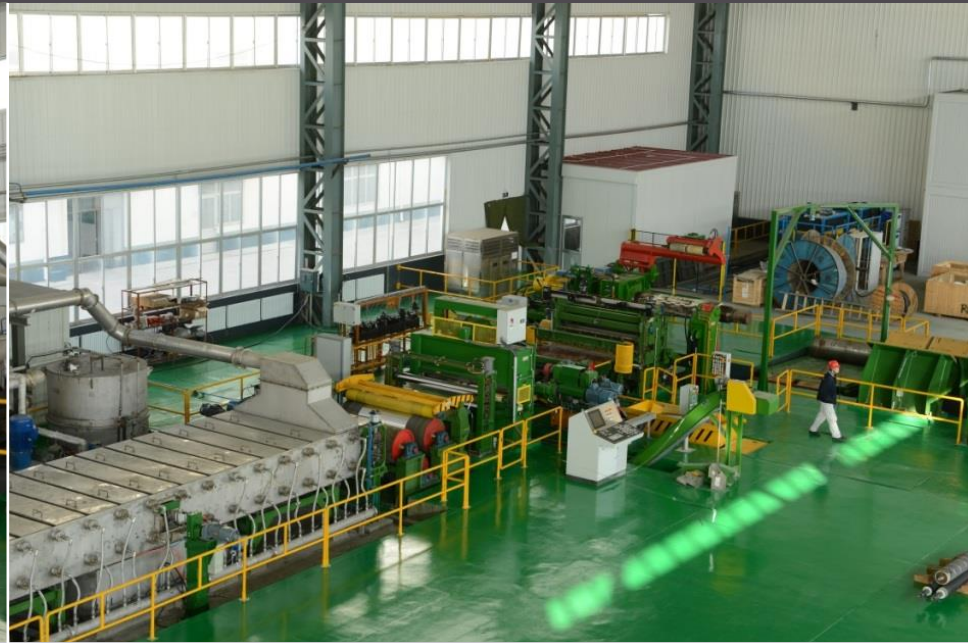
ENTRY SECTION AND CLEANING EQUIPMENT AT NANSHAN LIGHT ALLOYS
