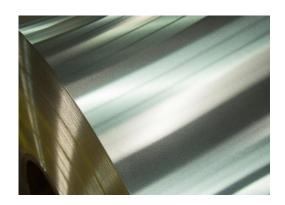
Aluminium strip produced with the innovative Alcoa Danieli Micromill process which offers improved mechanical characteristics: see possible production of 7xxx alloys to compete with steel.
