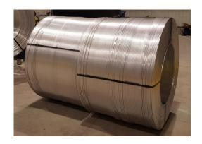
Endless aluminium hard-alloy rod production; less than 3 hours from ingot to finished coil with 3 operators.
